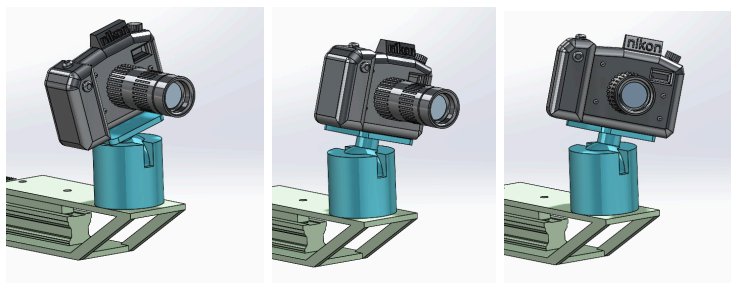
Figure 3.C.8. Camera Ball Joint Mount Positioning Motion.
