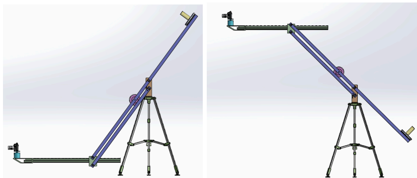
Figure 3.C.7. Max Arm Linkage and Fulcrum Up and Down Y-axis Motion (6 ft of motion).
