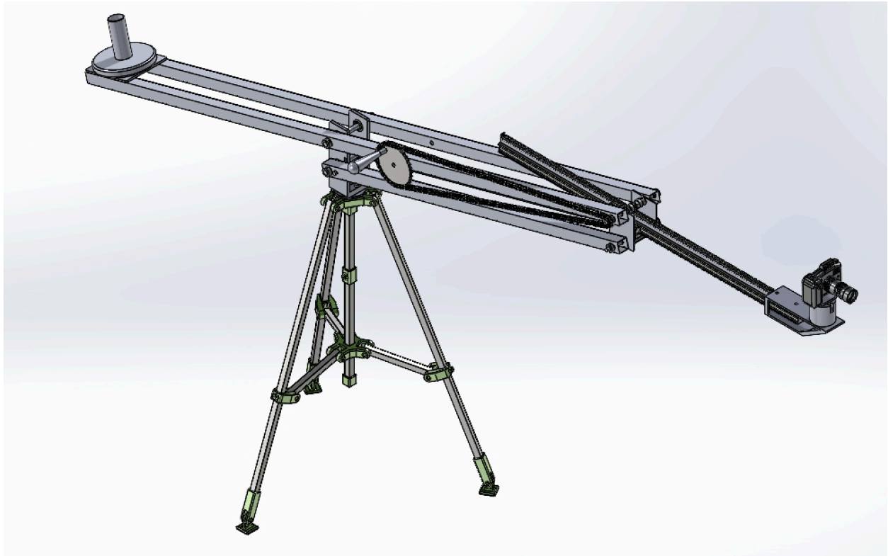
Figure 8.1. Final Detailed Design. Also depicted above are the tripod, counterweight, camera ball joint mount, and camera, which are sold separately.
